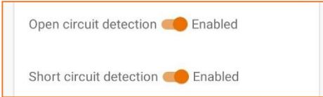
**Enable/Disable the Open Circuit function:** if a very small load is connected to the output of the dimmer, false open-circuits may be detected in some cases. In this case, it is recommended to disable the Open Circuit detection function.
